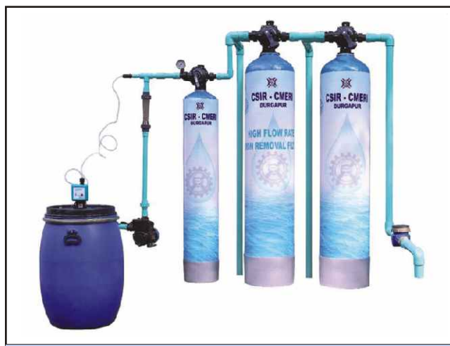
High Flow Rate Iron Removal Filter at CSIR-CMERI
