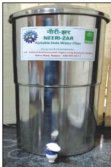
Household Unit (30 Lts capacity, Flow rate 10-15 Lts/hr.)
