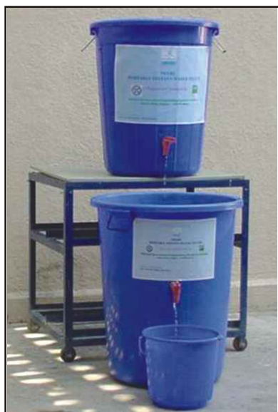
Community based Unit (200 Lts capacity, Flow rate 100-120 Lts/hr.)
