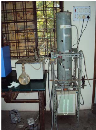
Bench scale bioreactor treating toluene and propanol
